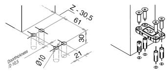
6. To install the floor plate, secure it in place with the screws provided as shown in the diagram.
