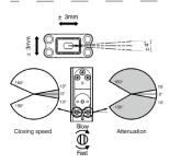
13. To adjust the closing speed and attenuation, turn the slots in the bottom pivot system. The placement of the floor plate can also be adjusted slightly.
