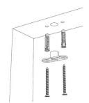
5. To install the top pivot system, cut a morticed hole into the top edge of
