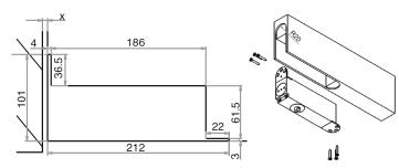
7. To install the bottom pivot system, cut a morticed hole into the bottom edge of the door panel as shown in the diagram. Place the bottom pivot system into the hole and secure it in place with appropriate screws.
