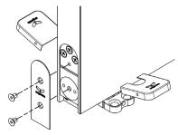
**15.** Attach the cover plates to the bottom pivot system and floor plate.
