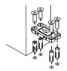
6. To install the floor plate, secure it in place with the screws provided as shown in the diagram.
