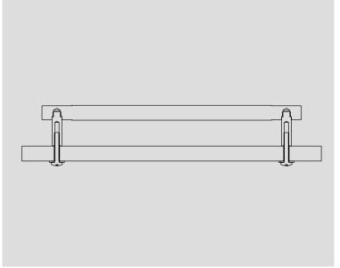
**4.** Ensure that you do not overtighten the screws. The washers should not bite in.
