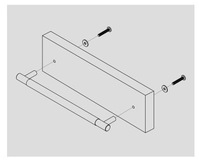
Hold the cabinet handle up so the legs align with the pre-drilled 5.5mm diameter holes.
