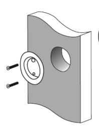
3. Secure the inside plate to the outside plate using the screws provided.
