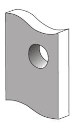
2. Drill a 54mm hole through the door. We recommend using a 54mm hole saw. For clean cut-outs, drill from both sides, meeting in the middle of the door.
