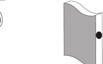
4. Fit the door edge finger pull by locating a position on the door edge approximately 150mm above the flush pull and drill a 25mm hole with a spade bit. Press in the finger pull. Use builders glue for a stronger fit.
