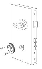
**15.** Fit the euro escutcheons around the cylinder on both sides of the door and fasten them with the wood screws provided.
