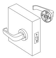
Note: The grubscrews may need a re-tighten after a bedding-in period. We recommend medium strength thread-lock to be used.
