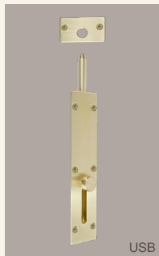
5225 Straight Throw > 105mm x 31mm > 9.6mm pin > 40mm throw > Custom lengths available
